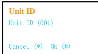
5. Press ID number to change the Unit ID. This is only necessary if you have more than 1 controller on a RS-485 bus.
